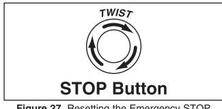
Figure 27. Resetting the Emergency STOP button.
